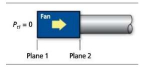
Fan static pressure is simply the losses in the system downstream of the fan, including the system's exit loss to atmosphere. This relationship may have led to the common practice of specifying fan static pressure instead of fan total pressure for fans installed in Installation Type B. Note that architectural louver ratings, when tested in accordance with AMCA 500-L, include exit losses from the building.
