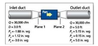
Note that at this point in the design process it's impossible to know whether the inlet or outlet duct areas match the fan's inlet or outlet, because in this hypothetical situation we are still in the process of selecting the fan. Because the duct must transition to the fan, the static pressures will change over the distance of the duct to the fan. This is a result of the velocity and velocity pressure changing due to the increasing or decreasing area of the transition.
