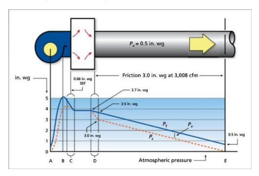
On the fan's outlet side, AMCA Publication 201 introduces the term "effective duct length." Effective duct length is 2.5 duct diameters when duct velocities are 2500 fpm or less, with one duct diameter added for each additional 1000 fpm. A centrifugal fan needs full effective duct length on its outlet to avoid system effect, while a vaneaxial fan needs 50% effective duct length. Fully developed flow is not needed to avoid system effect.
